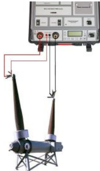
RMO-G cable connection on dead tank circuit breaker
